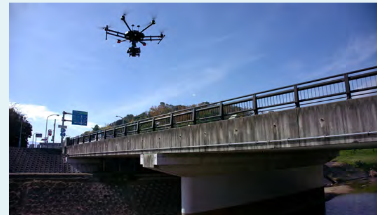
8K-camera drone on an aerial inspection
