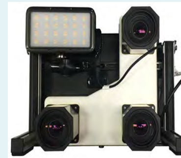
Triplet-lens camera rebar arrangement inspection system
